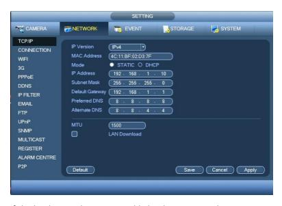
If the local network is DHCP-enabled, select **DHCP** in the **MODE** row, then click **APPLY** and then **SAVE** at the bottom right of the screen. Next, reboot the CVR/NVR.
