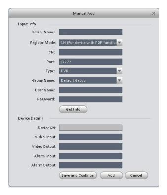
The **REGISTER MODE** needs to be set to **SN (FOR DEVICE WITH P2P).** The **DEVICE NAME** can be whatever you'd like to use. Just input the CVR/NVR's **SN** (see the image on pg. 7). Finally, enter your **USERNAME** and **PASSWORD.** (**Default is admin/admin**).
